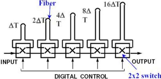
The variable time delay module selectively routes optical signals through N fiber segments having different lengths. Each fiber segment is defined to have the delay as
